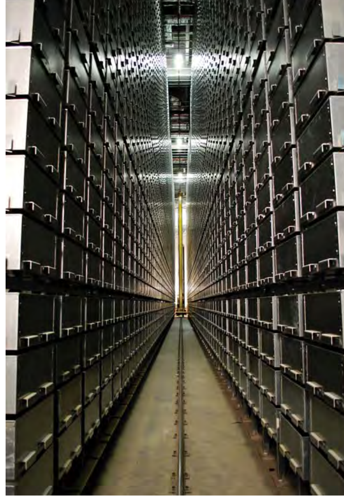
The underground automated storage and retrieval system in the Joe and Rika Mansueto Library. Photo by John Pitcher courtesy of the University of Chicago Library.
